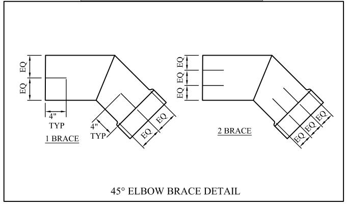
NOTE: BRACES HAVE 4-INCH LONG TACK WELD INSIDE RECTANGULAR END FOR ADDITIONAL STRENGTH
